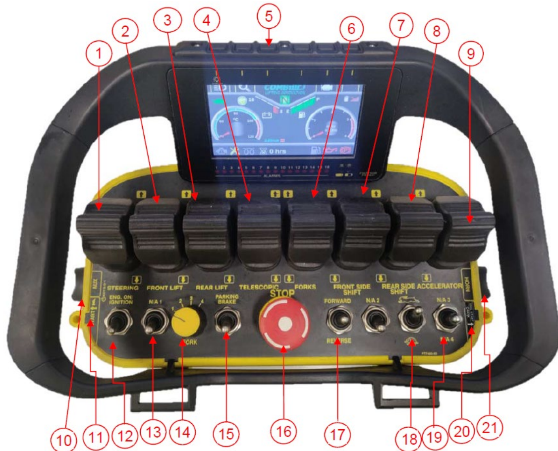
FIGURE 2.10 - REMOTE CONTROL LAYOUT TOP VIEW
