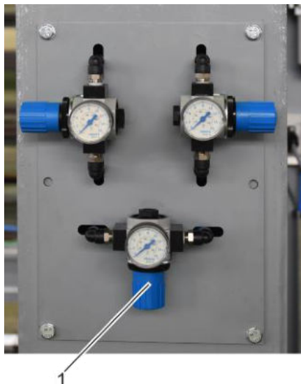
Fig. 33: Pressure regulator of the circumferential wire guide
