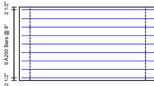
Bottom Slab Int. Reinf.
