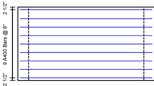
Bottom Slab Ext. Reinf.
